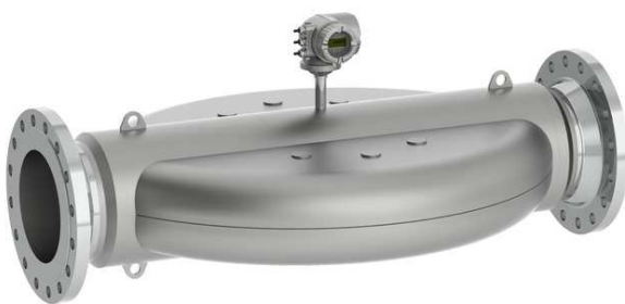
Fig. 2. Promass X : four tubes mass Coriolis meter with low uncertainty, extended usable turndown ratio and low pressure drop.
